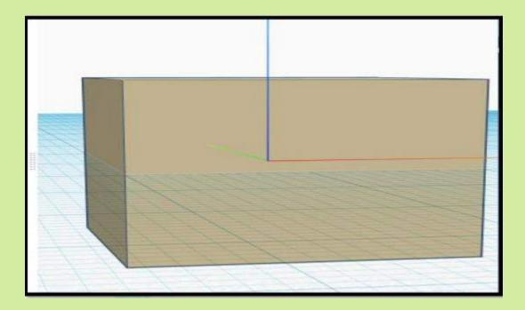
The coordinates icon is placed at the center point (X=0, Y=0, and Z=0) of the box shape. The X-axis (Width) is red, the Y-axis (Length) is green, and the Z-axis (Height) is blue. Note that half of the shape is below the workplane. How can we make a round hole in top of the box? Drag the Cylinder codeblock so that it snaps to the bottom of the Box codeblock. Expand it and set its Radius to 6. Press the Run button. I clicked-dragged the View-Cube (in the upper left) to get:
