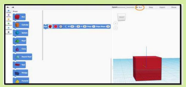
The general procedure is to make changes in a codeblock (such as the Add shape above) and press the Run button to see these changes rendered on the workplane. Press the red circle to change the color of the box. The gray-white button makes the box a "hole" (more on this below). The directional arrow is a toggle to expand/collapse the codeblock's variables and values. Replace the number zero in the Edge container and click on the Run button to see rounded edges on the box.
