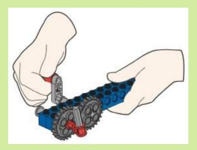
This model has a 1:3 gear ratio. The larger drive gear turns the smaller driven gear, resulting in increased speed, but reduced output force. This is called gearing up.
