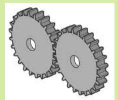
The drive gear is the gear that is turned by an outside effort, for instance your hand or an engine. Any gear that is turned by another gear is called a driven gear or follower. The drive gear provides the input force and the driven gear delivers the output force. Using a gear system can create change in speed, direction, and force. But there are always advantages and disadvantages. For example, you cannot have both more output force and an increase in speed at the same time.
