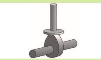
The profile of a cam allows it to control the timing and degree of movement of a follower. A cam can also be regarded as a continuous, variable inclined plane. Cams can be circular, pear shaped, or irregular.
