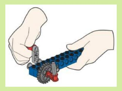
This model has a 1:1 gear ratio. The small middle gear is an idler gear. The idler gear does not affect the gear ratio, speed or output force of either the drive or the driven gears. The drive and the driven gears turn in the same direction and at the same speed.
