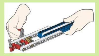
This model shows a differential gearing with a gear ratio of either 28:20 or 7:10. The input force is transferred to two output forces at an angle of 90°. When one output pointer is stopped the other will double its original speed. When both output pointers are stopped the handle cannot be turned.
