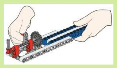
This model shows a rack and pinion gearing. Unlike the previous gears a rack and pinion gearing can only be used for linear motion, not rotary. When the handle is turned the gear rack moves forward or backwards depending on the rotational direction of the small gear (called a pinion).
