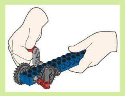
This model shows a gearing set up for periodic movement e.g. the driven gear turns for a short while then stops for a moment. Speed is significantly reduced, as movement only occurs when the driven gear is meshed with one of the two drive gears.
